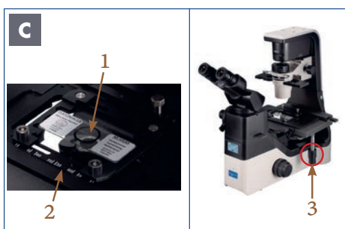
Illustration 055 C: NIB630 - Place sample on the mechanical stage.
