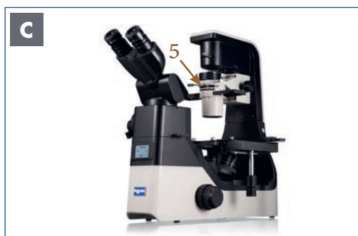
Illustration 061 C: NIB630 - Observation with emboss contrast.
