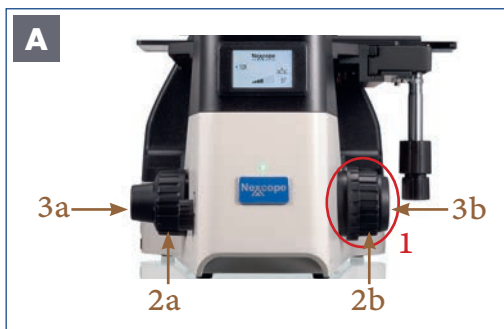
Illustration 045 A: NIB630 - Focusing controls.
