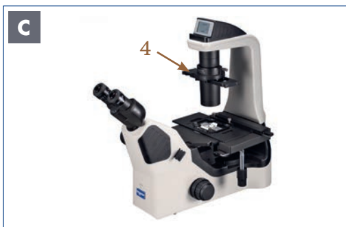
Illustration O60 C: NIB610/NIB620 - Observation with emboss contrast.
