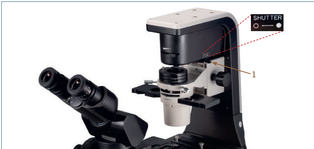
Illustration O48: NIB630 - Transmitted light path shutter.
