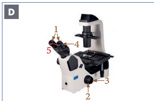
Illustration 028 D: NIB610/NIB620 - Settings on the observationtubus.
