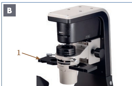
Illustration 055 B: NIB630 - Adjustment of the phase contrast slider.
