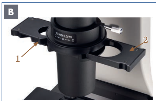
Illustration 028 B: NIB610/NIB620 - Settings on the condenser.
