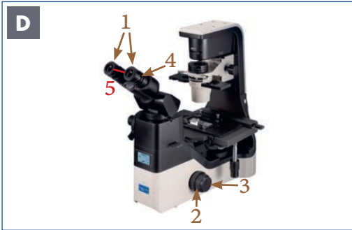
Illustration 055 D: NIB630 - Settings on observationtubus.
