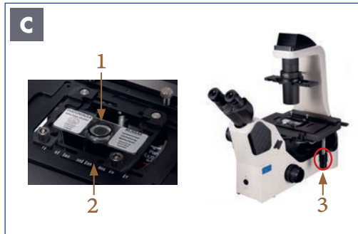
Illustration 028 C: NIB610/NIB620 - Sample placement.
