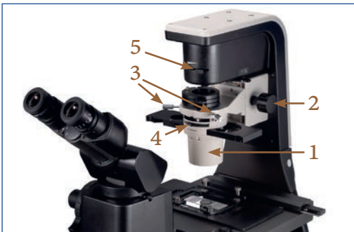
Illustration 052: NIB630 - Components of the Koehler illumination.
