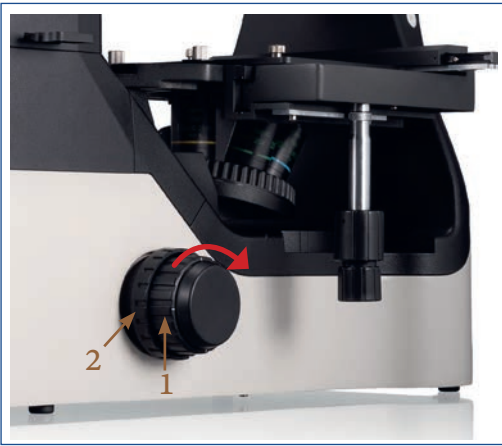
Illustration 046: NIB630 - Tension adjustment ring.
