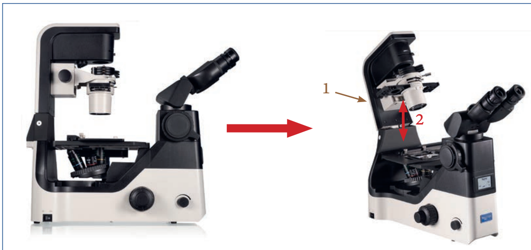
Illustration O49: NIB630 - Tiltable lightning unit.
