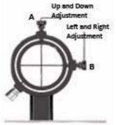
Loosen the finder bracket lock thumbscrew on the telescope.
