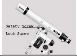
First tighten the dovetail lock screw, and then tighten the small chrome safety screw onto the dovetail mounting block until snug.
