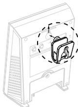
Place a screw on the wall where you wish to hang for sensor. Hang the sensor on to the screw with or without the mounting adaptor.
