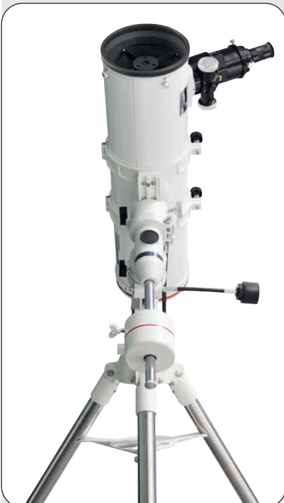
Fig. 16b: The polar home position, front view.
