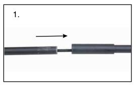
Connect 3 section of steel tubes by inserting them to each other. The tubes are spring loaded in-series. The length should be about 2.8 meters.
