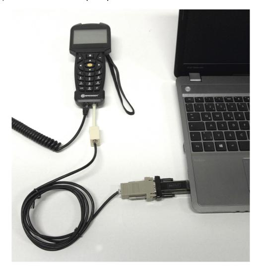
**NOTE:** Short white cable adapter to be used only for uploading process!
