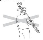
Remove camera and other equipment from the tripod while transporting. Camera or other equipment may fall from the tripod and cause bodily injuly or property damage.
