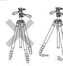
To prevent accidental equipment fall or tripod tipping over, making sure all levers, knobs and handles on the unit are securely tightened.
