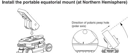
Rotate wedge mounting dial to mount the wedge to the main body.
