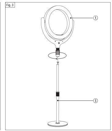
Step 2 :Screw the ring light with the fork arm (1) on top of the stand (5).
