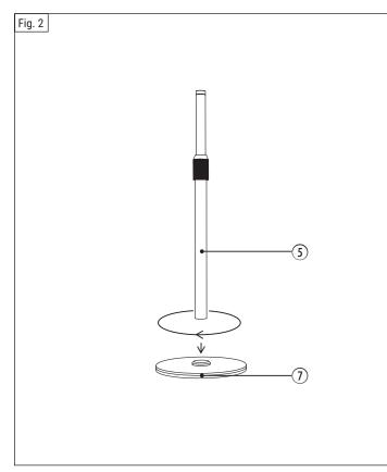
**Step 1** :Screw the stand (5) into the base plate (7).
