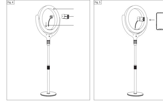
**Step 3:** Insert the flexible arm (2) into the ring light (1). Press the smartphone holder (10) into the ball joint of the flexible arm (2).
