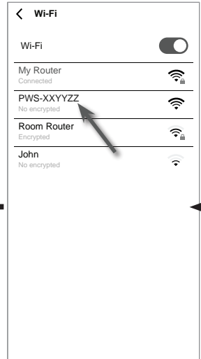
(d) Select the console WI-FI network name (the name always begin with PWS-) to connect your smart phone to the console. Then tap back to WSLink app.
